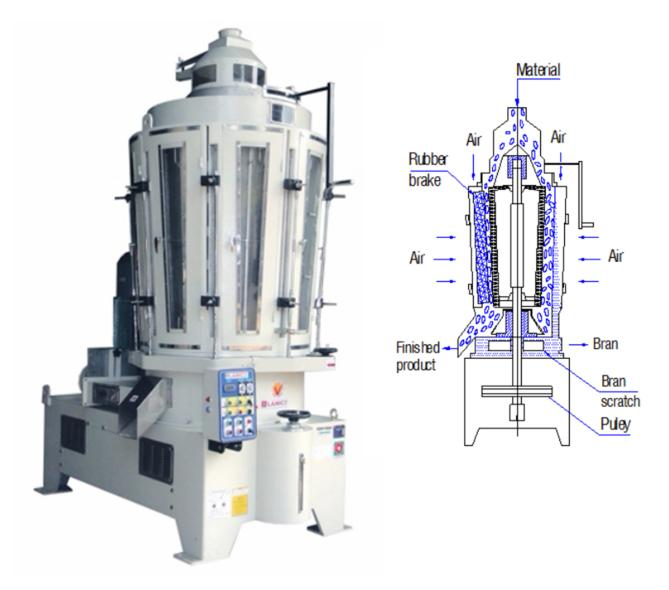
Rice Whitener is designed basing on a friction between rice-screen-abrasive stone (it's section profile is cone cylinder) combining with rubber bar to take off a thin bran on surface of rice. In the mean time, air pressure is put directly into the gap of stone and screen so bran is taken out ultimately, finished rice is cool and without bran.
